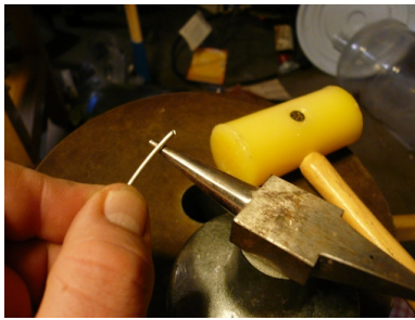
(b) Bending the pin on an anvil.
