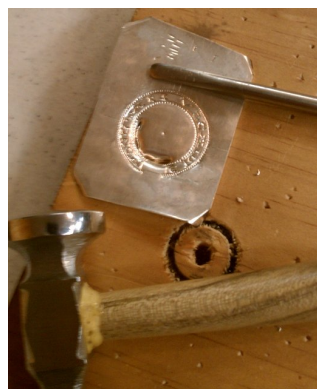
(g) Cutting out the brooch with a chisel, interior.
