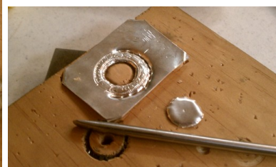
(h) Cutting out the brooch with a chisel, exterior.
