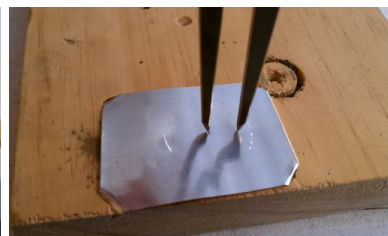
(b) Scribing guidelines with a compass.
