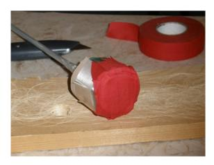
Using a neutral colored tape (black cloth tape or duct tape) cover the rest of the head. Continue this wrap down onto the shaft, placing another layer of tape over the strapping tape which adhered the foam to the blunt and shaft. You can either spiral down with one continuous piece, or cut separate pieces of appropriate lengths. A 2" wide roll of tape is very useful for this step.
