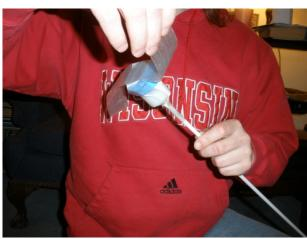
Using this same width of strapping tape, cut a piece that will wrap several times around the shaft (about 3 times around is good, which should be ~4") Near the base of the blunt, wrap this tape tightly around the shaft and other pieces of strapping tape. It will pull the strapping tape "x" tightly onto the foam and blunt, and will prevent the head from moving on the shaft.
