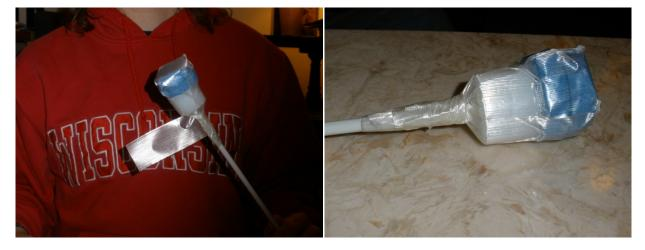
Cut pieces of craft foam that are between 1  $\frac{1}{2}$ " and 2" wide. We use 1  $\frac{1}{2}$ ". It must be wide enough to extend from the front of the foam head to at least  $\frac{1}{2}$ " over the UHMW blunt. Wrap
