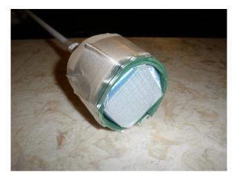
Place a layer of strapping tape covering the entirety of the exposed region of the shaft (from the base of the APD to where the strapping tape already covers it by the head.) We use a 1" wide piece, cut to the length of the exposed shaft (~24"), and carefully roll it on. Make sure the entire shaft is covered, as the strapping tape will prevent any splinters from breaking off if the shaft should receive enough of a blow to break it.
