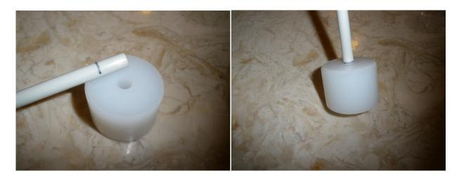
Drill a 1/16" hole in the side of the Asgard APD. This should enter the cavity that the shaft will go in to, and is placed near the bottom of the nock. The purpose of this hole is to allow for excess glue and air to squeeze out when the shaft is attached.
