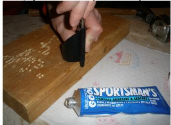
Place the APD on a board, with the nock hanging off the edge and pointing down. Make sure the board is on a sturdy surface. Place the shaft into the glued cylinder, and use a mallet to pound it into place. As the shaft goes into the APD, glue will squeeze out of the hole – you will want to have a paper towel/newspaper covering any surface you do not want to become glue-covered.
